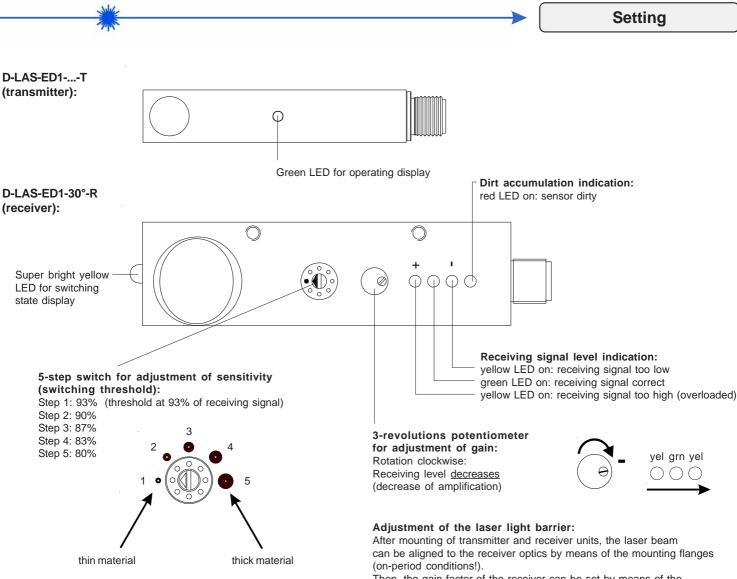
Then, the gain factor of the receiver can be set by means of the potentiometer, the optimal gain is indicated via the green LED.
