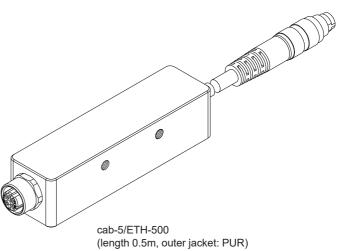
cab-5/ETH-500 (length 0.5m, outer jacket: PUR) 4-pole M12 fem. conn. (D-coded) for connection of an external CAT5 cable, e.g. cab-eth/M12D-RJ45-flx-(length)
