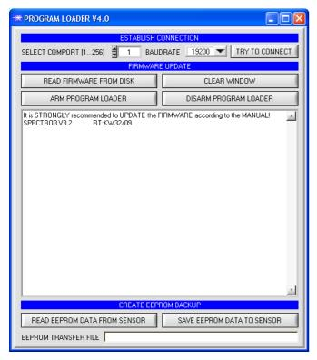
The software "Program Loader" allows the user to perform an automatic firmware update. The update will be carried out through the RS232 interface.
