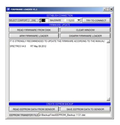
The software "Firmware Loader" allows the user to perform an automatic firmware update. The update will be carried out through the RS232 interface.
