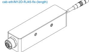
cab-4/ETH-500 (length 0.5m, outer jacket: PUR) 4-pole M12 fem. conn. (D-coded) for connection of an external CAT5 cable, e.g. cab-eth/M12D-RJ45-flx-(length)
