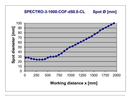
Relative intensity 100% SPECTRO-3-1000-COF-d50.0-CL: 100% at a working distance of 860 mm (INTENSITY 3666)
