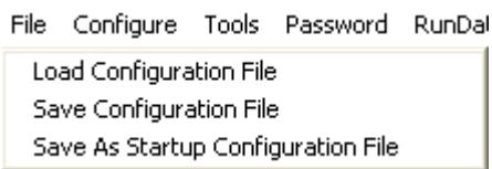
In the "File" menu, configuration files that are set under "Configure" can be saved to a file or loaded from a file. The "Save As Startup Configuration File" item defines the currently set parameters as startup parameters, i.e. these parameters will be loaded automatically when the software is started.
