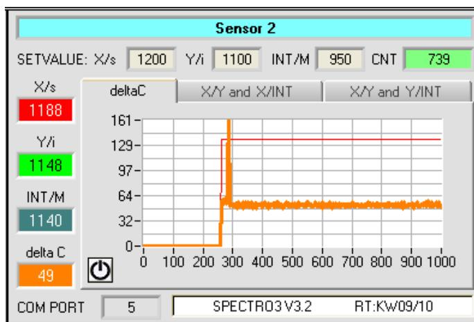
Data immediately are saved in the corresponding created file, if it is activated, and visualised on the user interface. The total number of recorded values is displayed in the **CNT** field.
